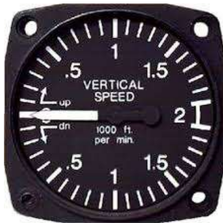
Figure 1.8 Vertical Speed Indicator
